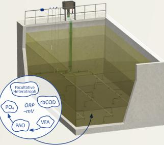
A longer anaerobic SRT combined with a lower **ORP** environment increases VFA production, enhancing biological phosphorus removal. VFAs are transported throughout the reactor via intermittent pulses of mixing without disrupting the fermentation layer.
