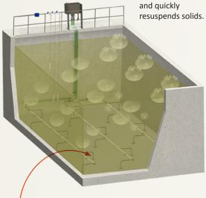
Nozzles near the floor of the tank release short bursts of compressed air, providing effective mixing.
