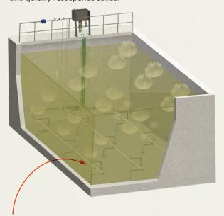
Nozzles near the floor of the tank release short bursts of compressed air, providing effective mixing. Periods of mixing are important to homogenize the substrate and microorganisms.
