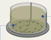
Headers follow the contour of the floor, eliminating dead zones that are created beneath conventional systems.
