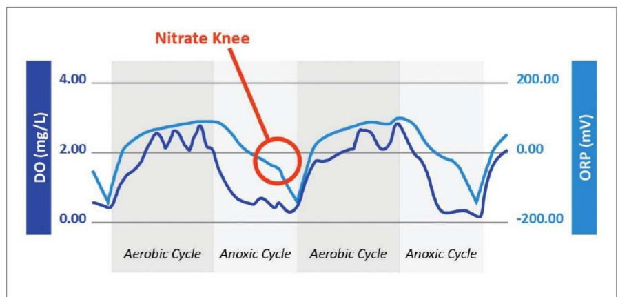
Figure 6. Transition from anoxic cycle to aerobic cycle using low ORP setpoint and nitrate knee.
