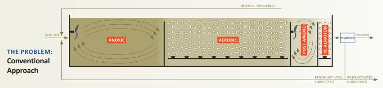
**Fixed anoxic and aerobic volumes** are designed for a single future state condition, offering **limited flexibility** for all other operating conditions.
