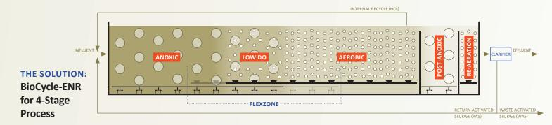
Without fixed baffle walls, FlexZone enables the anoxic, low DO, and aerobic volumes to expand and contract as operating conditions and kinetics change, ensuring effluent quality compliance.
