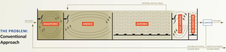
**Fixed anaerobic, anoxic, and aerobic volumes** are designed for a single future state condition, offering **limited flexibility** for all other operating conditions. Conventional point source mixers **require physical baffles** to facilitate the mixing regime needed to ensure complete mixing.
