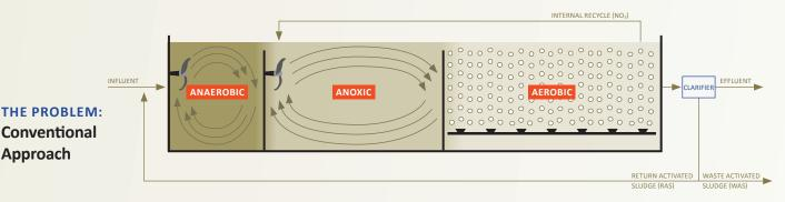
**Fixed anaerobic, anoxic, and aerobic volumes** are designed for a single future state condition, offering **limited flexibility** for all other operating conditions. Conventional point source mixers **require physical baffles** to facilitate the mixing regime needed to ensure complete mixing.
