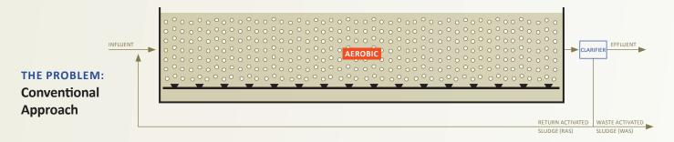
**Fixed aerobic volumes** are designed for a single future state condition, offering **limited flexibility and lack of process control**.
