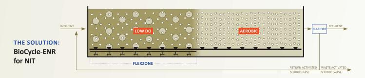
The FlexZone enables low DO and aerobic volumes to expand and contract as operating conditions and kinetics change, ensuring effluent quality compliance while minimizing energy consumption.
