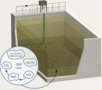
A longer anaerobic SRT combined with a lower ORP environment increases VFA production, enhancing biological phosphorus removal.
