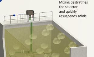
Nozzles near the floor of the tank release short bursts of compressed air, providing effective mixing. Periods of mixing are important to homogenize the substrate and microorganisms.
