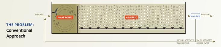
**Fixed anaerobic and aerobic volumes** are designed for a single future state condition, offering **limited flexibility** for all other operating conditions.
