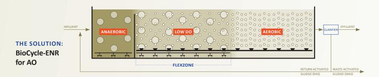
The FlexZone system enables the low DO and aerobic volumes to expand and contract as operating conditions and kinetics change, ensuring effluent quality compliance.
