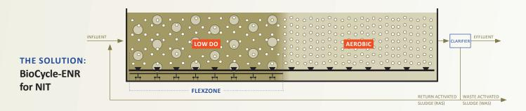
The FlexZone system enables low DO and aerobic volumes to expand and contract as operating conditions and kinetics change, ensuring effluent quality compliance while minimizing energy consumption.
