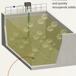
Nozzles near the floor of the tank release short bursts of compressed air, providing effective mixing.
