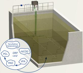
A longer anaerobic SRT combined with a lower **ORP** environment increases VFA production, enhancing biological phosphorus removal. VFAs are transported throughout the reactor via intermittent pulses of mixing without disrupting the fermentation layer.
