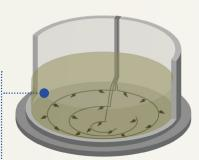
Effective aeration and mixing with no minimum depth requirements.
