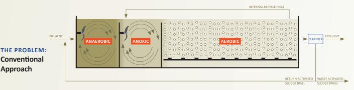
When operating at less than design conditions, excess aerobic volume leads to high DO in the internal recycle and RAS streams, negatively affecting denitrification and biological phosphorus removal.
