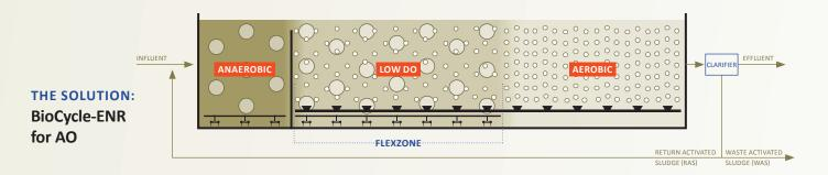
The FlexZone system enables the low DO and aerobic volumes to expand and contract as operating conditions and kinetics change, ensuring effluent quality compliance.
