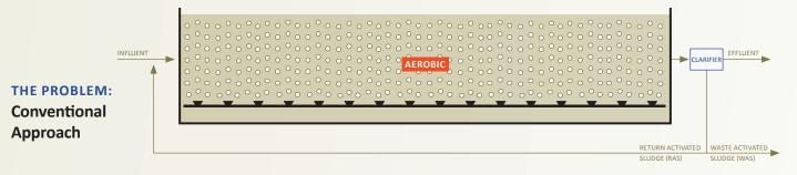
**Fixed aerobic volumes** are designed for a single future state condition, offering **limited flexibility and lack of process control**.
