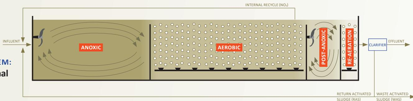
Stringent effluent nitrogen limits can require high internal recycle (IR) pumping rates.
