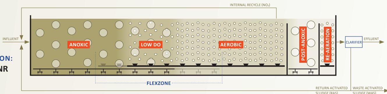
Extra capacity is operated as a low DO environment for **simultaneous nitrification and denitrification**, resulting in lower IR pumping rates.
