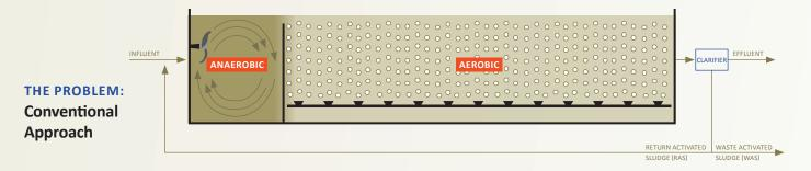
**High nitrate concentrations in the RAS stream** can alter anaerobic conditions and inhibit biological phosphorus removal.
