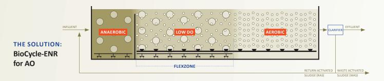
**SyncroMix**, the unique combination of BioMix integrated with fine bubble diffused aeration, **creates low DO environments** and prevents mixing limited over-aerated conditions through **independent control of aeration and mixing**.
