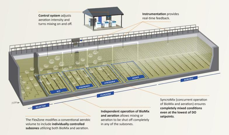
Utilizing complementary mixing patterns and eliminating the need for separate tanks or baffle walls, the FlexZone dynamically adjusts subzone operation to address changing conditions.
